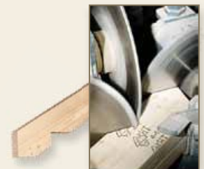
Accurate machine cut rafters make a tight joint for maximum strength and precise construction.
